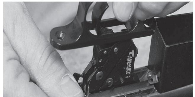
8) Install the bolt in the barreled action and check trigger function and safety function.
