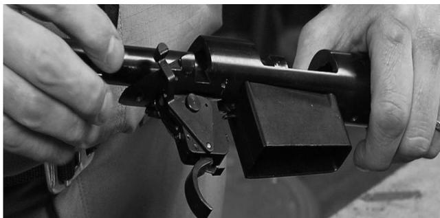
9) With an empty chamber or with Snap Caps installed, with the safety lever on Safe, pull the trigger. The firing pin should not move.
